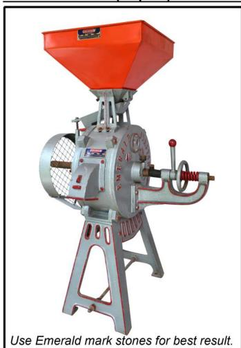
**Emerald Danish Model Mills** popular modal are export. The mills body is made from full Cast iron. Emerald mills are fitted with Grain hopper, Grain feeder, dust proof bearing housing & bearings, bright shaft, safety Springs, Fines Control device with momentary disengaged system Flour out let and stand. The mills are suitable to grind all kind of Food grains.
